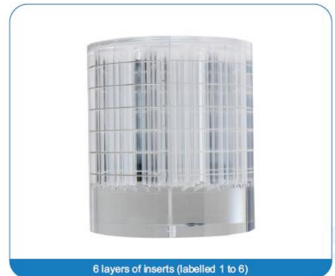
7 insert columns (6 peripheral, 1 central)
